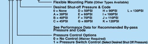
2 = Pressure Relief Valve (Select Recommended By-Pass Pressure)
